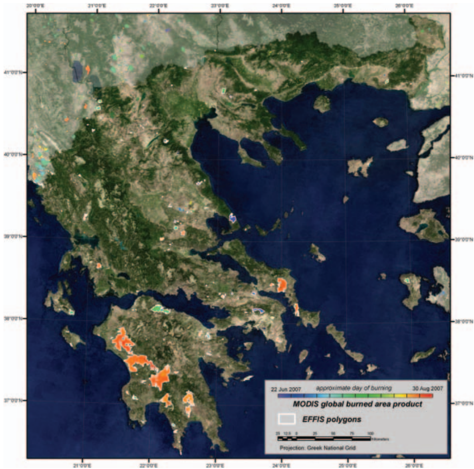
Figure 1. Map of the extent burned and approximate day of burning in Greece mapped by the MODIS burned area product for 22 June to 30 August 2007 with white vectors superimposed showing the burned areas mapped independently by the European Forest Fires Information Service (EFFIS). See text for further details.
